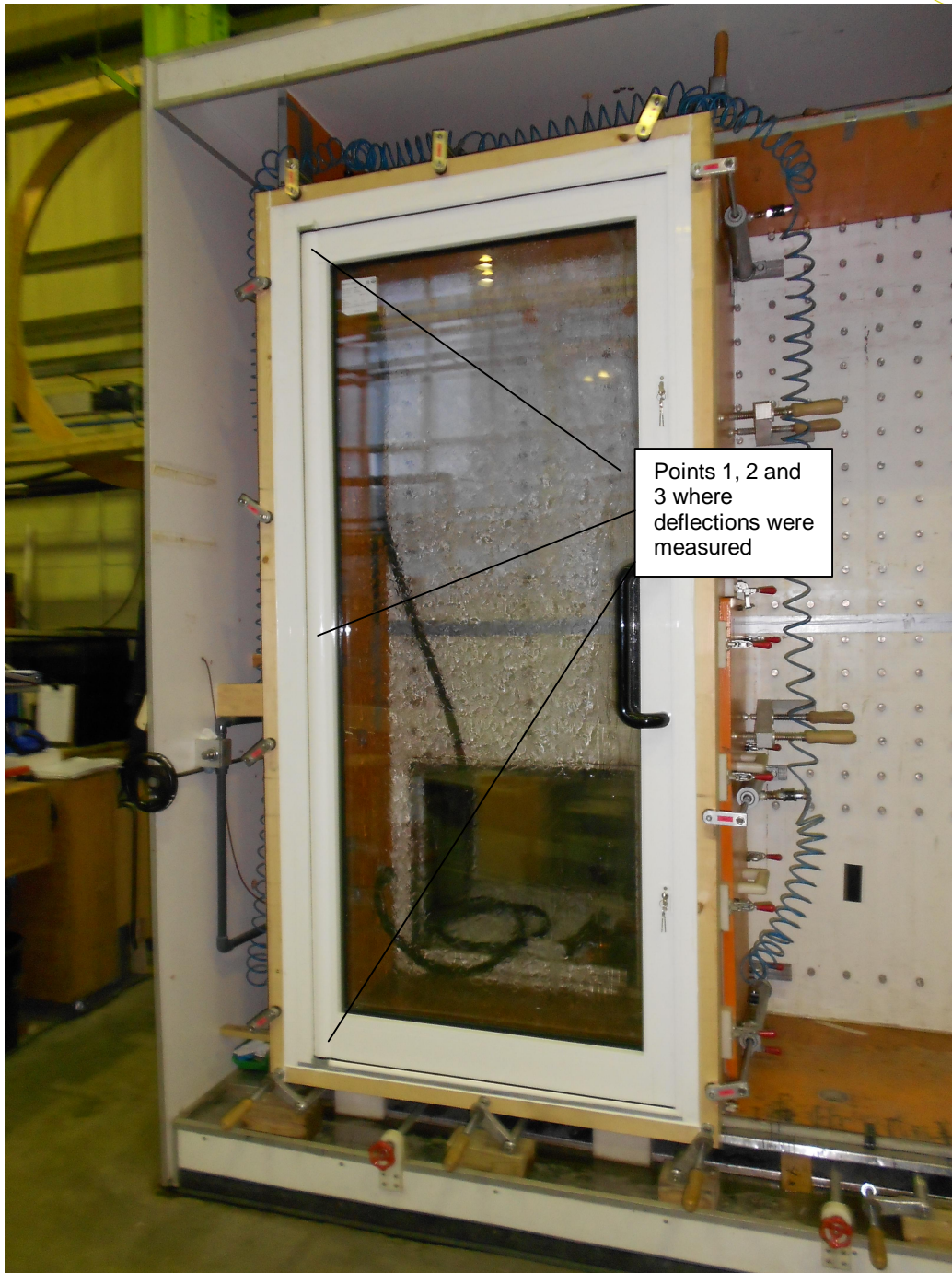
Figure A3. The test specimen showing points 1, 2 and 3 where deflections were measured.
