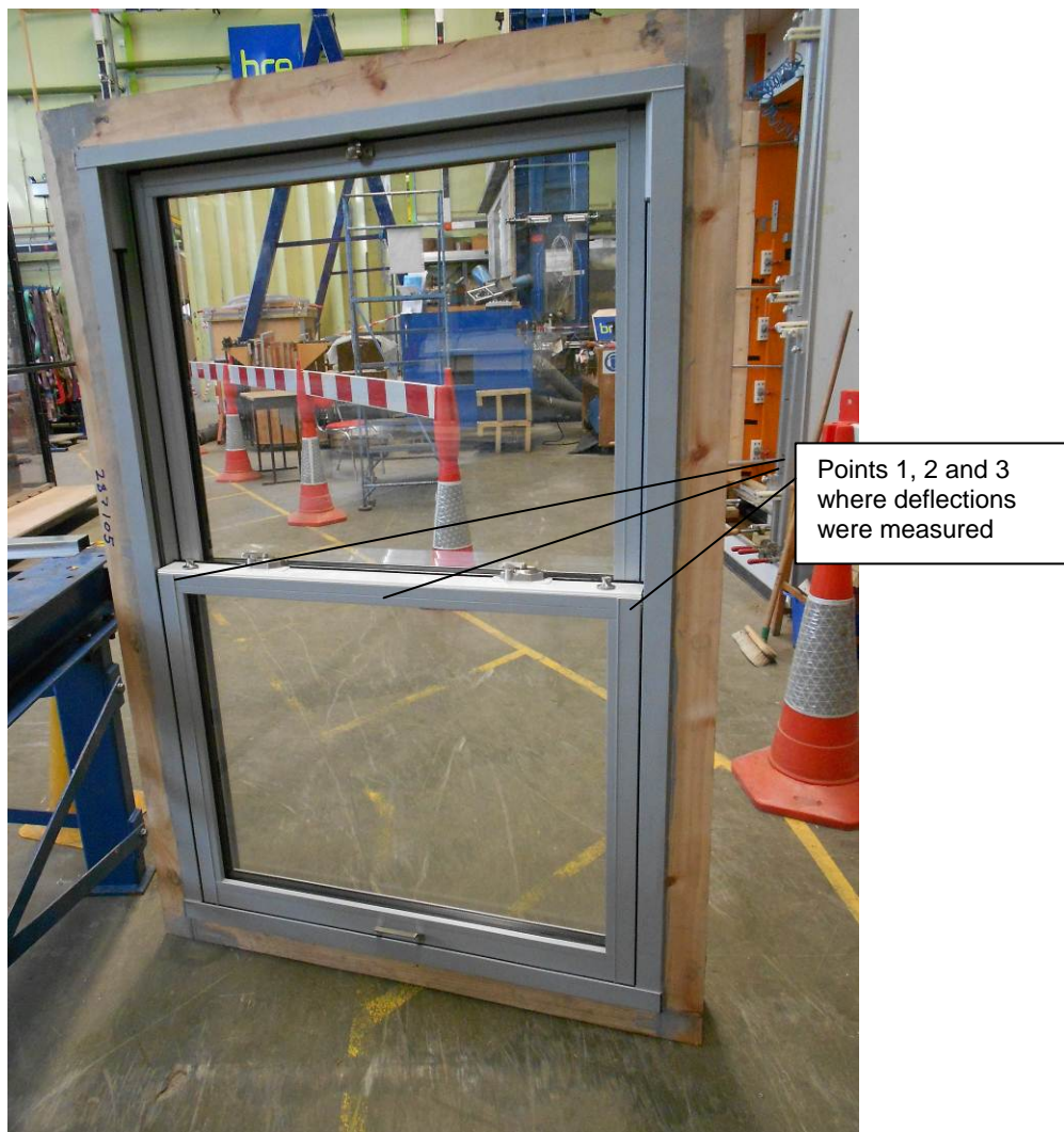
Figure A2 The test specimen – indoor face showing points 1, 2 and 3 where deflections were measured
