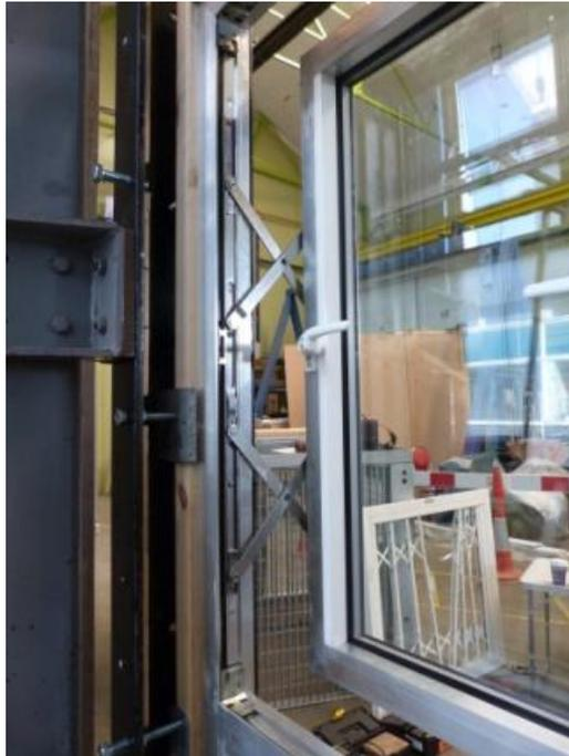
**Figure 6** Locking system keeps
