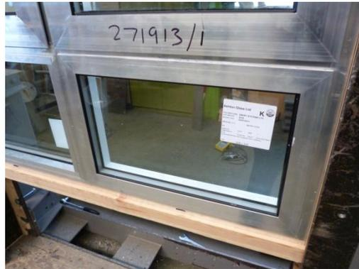
**Figure 10** Externally glazed light viewed from non-attack side
