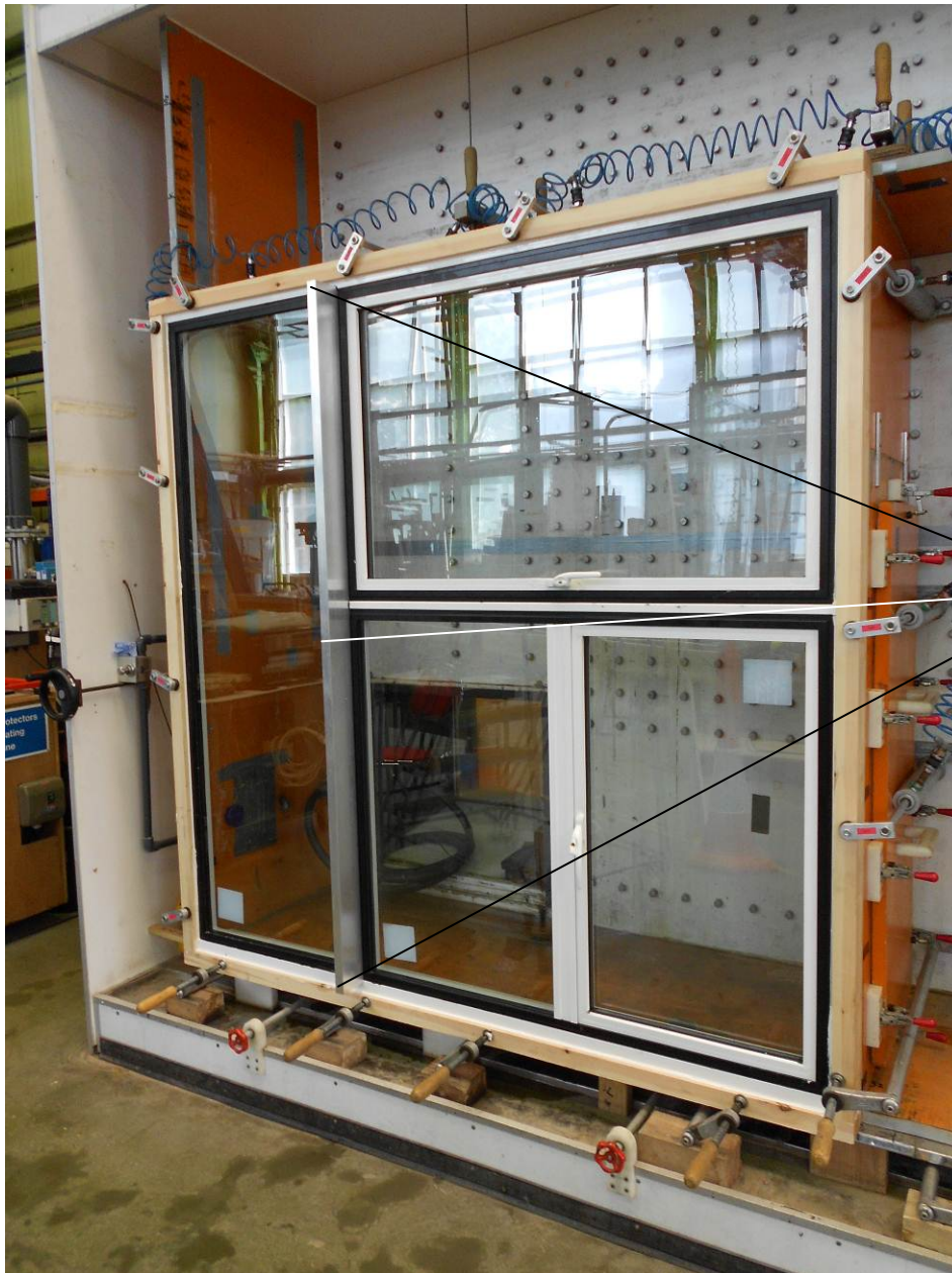
Figure A3 The indoor face of the test specimen showing points 1, 2 and 3 where deflections were measured
