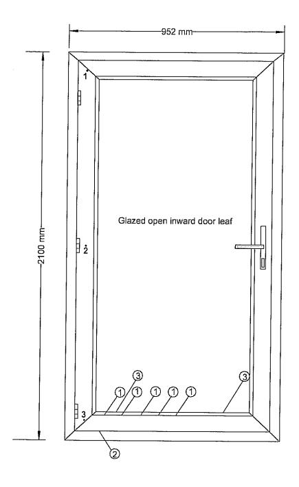
Figure 1. Outline sketch of the inside face of the door showing positions of deflection measurement points (on left hand stile) and points where water leaked through the door at 250 and 300 Pa test pressures
