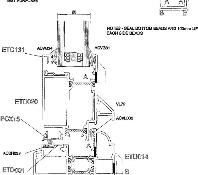
Drawing showing a cross section of frame members at the base of the door
