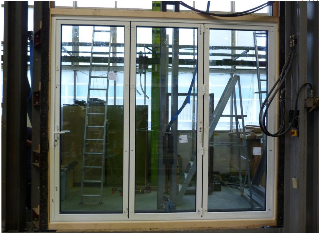
Figure 2 Internal face of folding doorset
