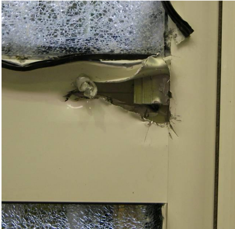
Figure 6 Result of attempting to lever the mid-rail profile
