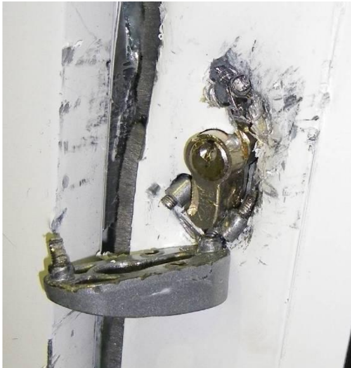
Figure 14 Cylinder exposed during attack test 25
