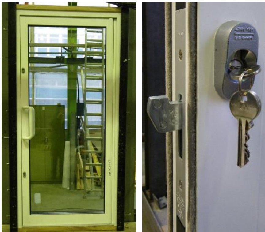
Figure 1 Specimen 260634/01 mounted in BRE test rig, and detail of upper hook lock and escutcheon (lower hook lock was oriented in opposite direction)
