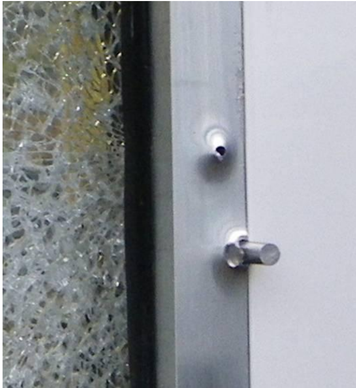
Figure 5 Punches penetrating through beading
