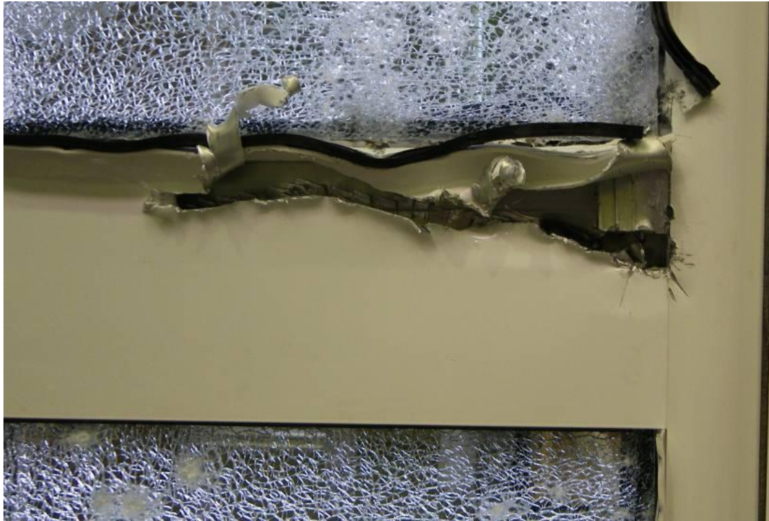
Figure 7 Result of second attempt to lever out the mid-rail profile
