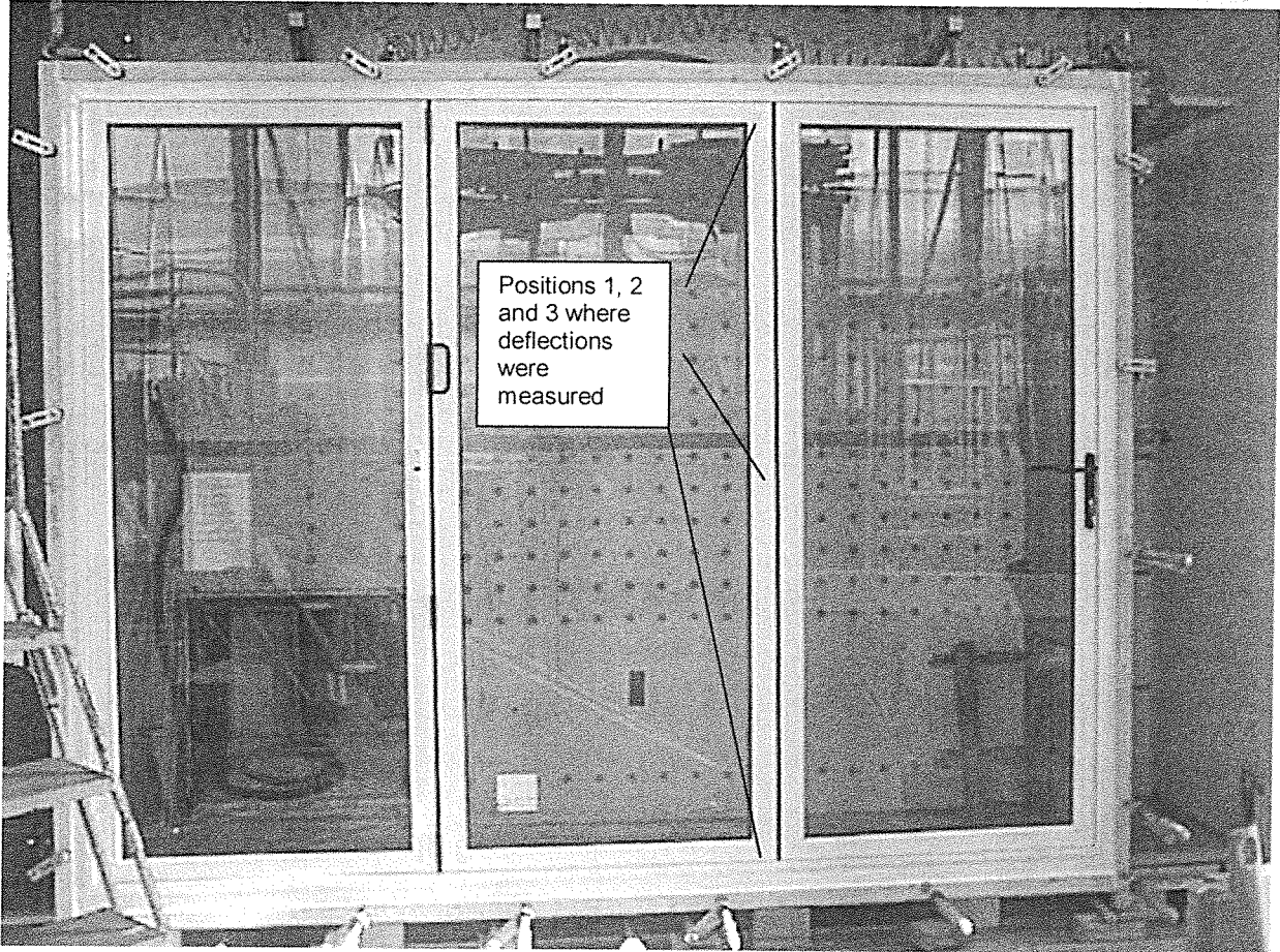
Figure A3. Smart Systems Visofold 1000 door showing points where deflections were measured
