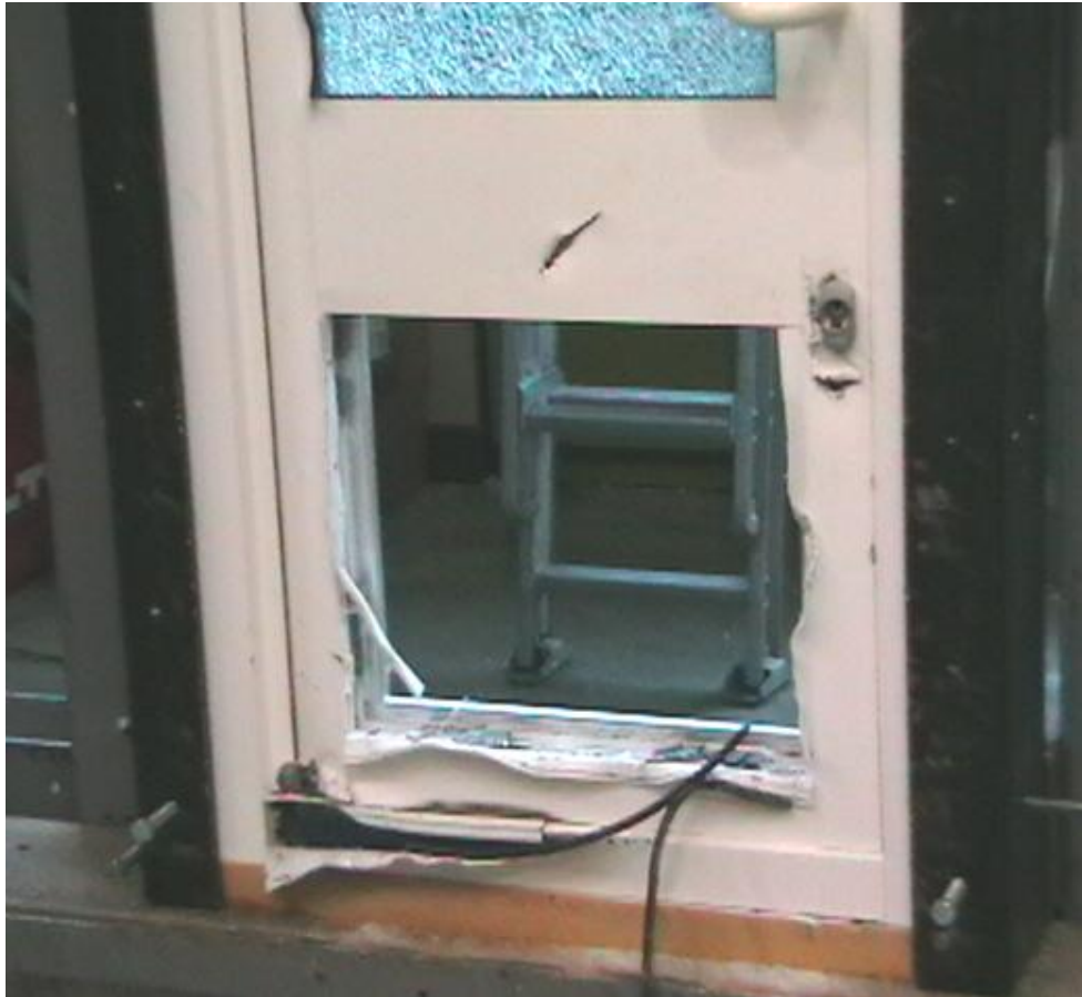
Figure 10 Damage sustained by the lower glazing panel on specimen 260634/02 during burglary test 5
