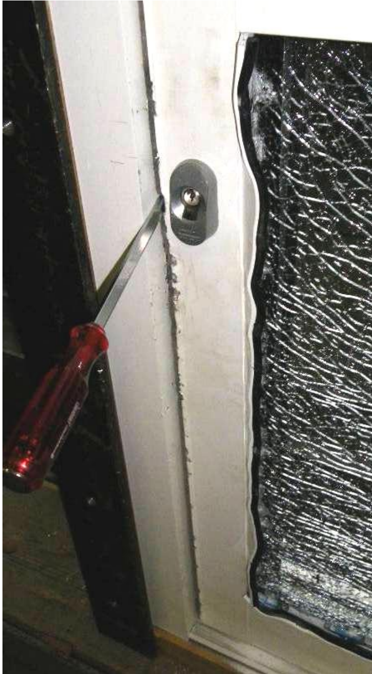
Figure 8 Damage sustained by the leading edge of the door leaf on specimen 260634/03 during burglary test 2
