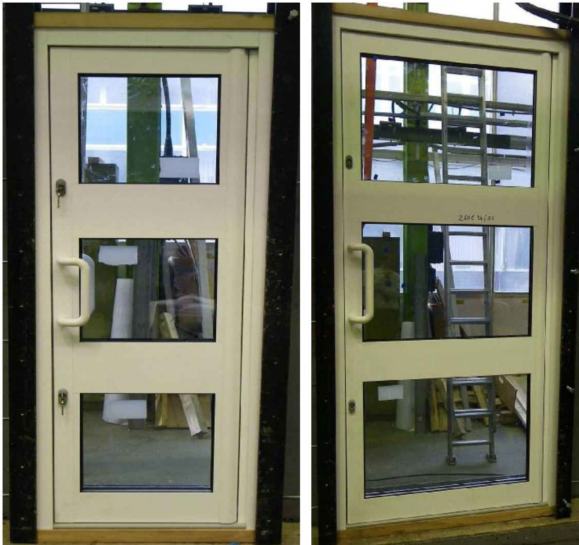
Figure 2 Specimen 260634/02 (left) and 260634/03 (right) mounted in the BRE test rig
