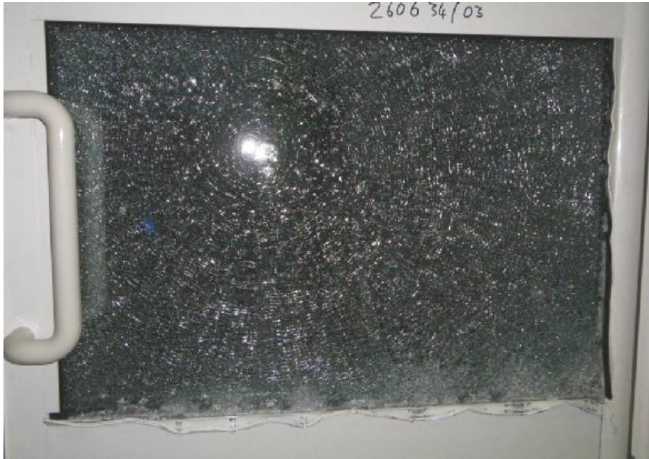
Figure 9 Damage sustained by the door leaf around the central glazed infill panel on specimen 260634/03 during burglary test 4
