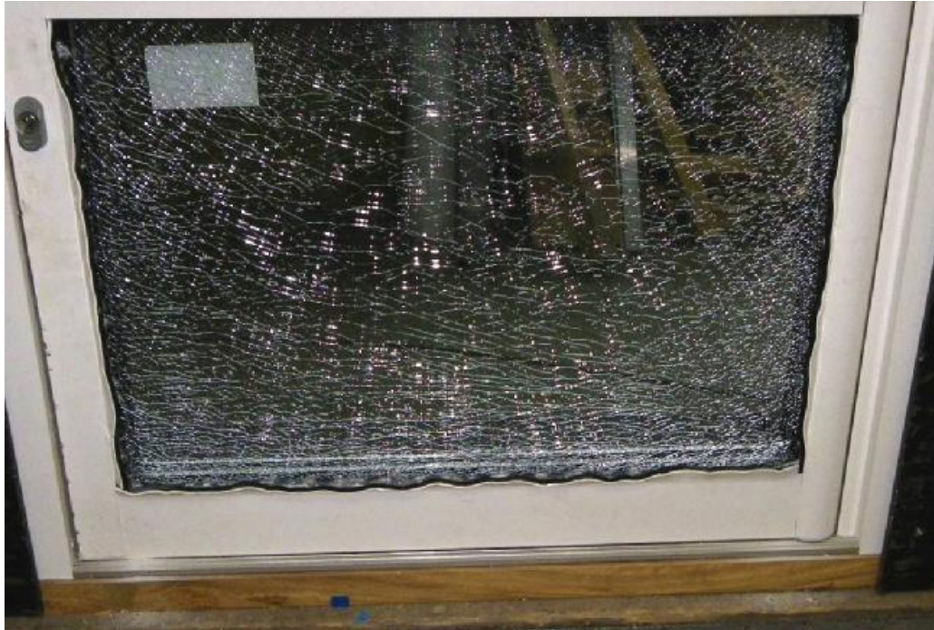
Figure 7 Damage sustained by the door leaf around the glazed infill panel on specimen 260634/03 during burglary test 1
