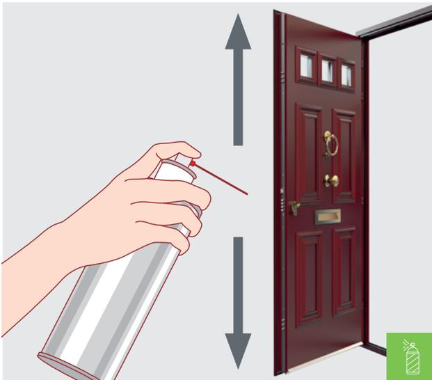
5. Spray the light engineering oil around the door pins (starting at the top of the door and working your way downwards). 2-3 seconds is enough spray time.
