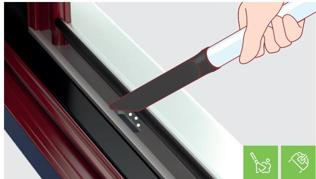
4. Use a small brush to loosen any debris from the drainage slots and then vacuum away the dirt.
