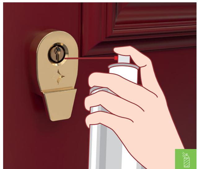
4. Spray the light engineering oil into the escutcheon (key hole) and insert the door's key a few times to ensure easy operation. Use as much lubricant as you can without it pooling in the door lock or handle.
