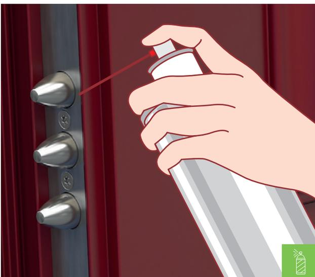
3. To clean the lock, lubricate around the pins using a light engineering oil (an aerosol spray with a straw is ideal). This will allow you to make sure that the oil penetrates deep within the locking mechanism.
