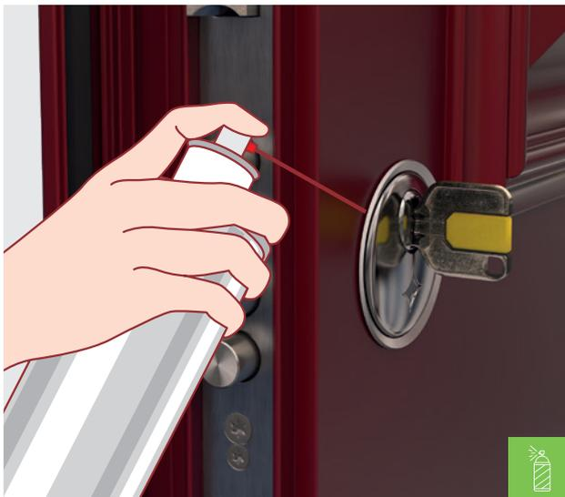
7. After cleaning around the lock pins, immediately re-apply the light engineering oil to lubricate the lock and replace the lubricant that was removed during cleaning.
