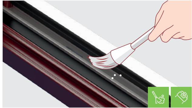
2. Use a small brush (a paint brush is ideal) to loosen any debris from the threshold and then using a vacuum, remove the dirt that has been collected.
