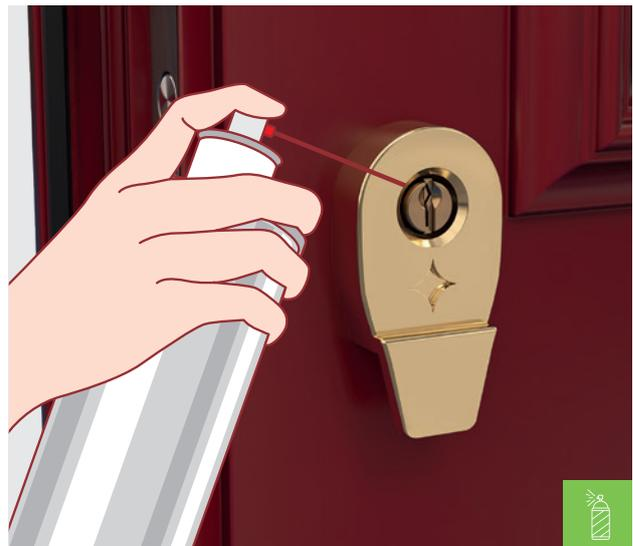
8. Similarly, after cleaning the escutcheon, replace the lubricant that has been cleaned away by re-applying the light engineering oil.
