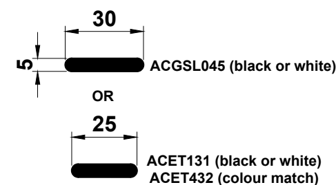
Drainage Through Vent
